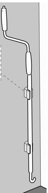
**EN** If you want to fasten the support legs to the vehicle (optional fixing), fix the wall brackets (only on reinforced points).
