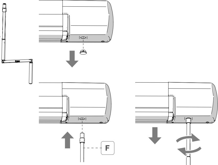
**EN** In case of engine failure, use crank handle **F** delivered as standard.
