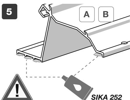
**EN** **Important:** use of SIKA 252 adhesive is essential for fixing the bracket (brackets).
