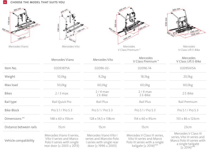
\* This version allows the installation of the rail support base in two different positions, one standard and one lower to make it easier to load the bikes. Lower version must be used with the License Plate Carrier, which has the license plate holder bar and regulation lights.
