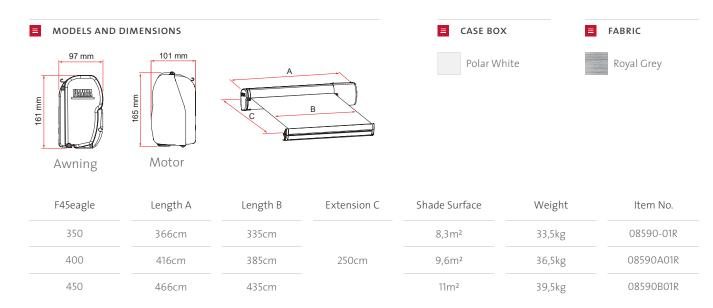
Important: verify with your trusted dealer if your motorhome or motorcaravan is suitable for the installation of the F45eagle with sturdy full length aluminium bracket. The vehicle must be robust enough to support the weight and the tension of the open awning. Fiamma refuses all responsibility for damages to the walls or for water ingress due to incorrect installation or due to installations on weak walls.
