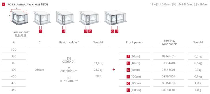
[S] and [L]: complete with magnet kit (2 sets of 6 magnets) which, inserted in the side panel pocket, permit complete adhesion to the Ducato vehicle. \*\* This model is suitable for vehicles with straight wall, height from ground 245-280cm.
